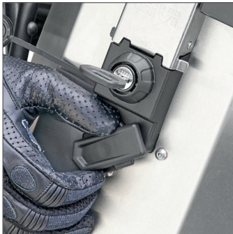
The cases are detached from the side frame by turning an external knob that is equipped with a cable system (patent pending).
