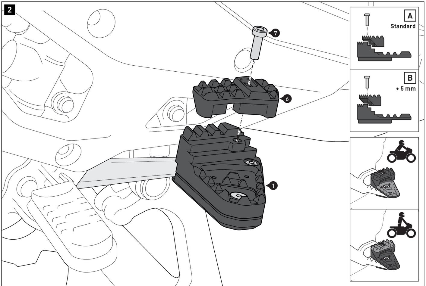
Screw the riser (6) onto the extension (1) in position [A] (standard) or [B] (+ 5 mm).
