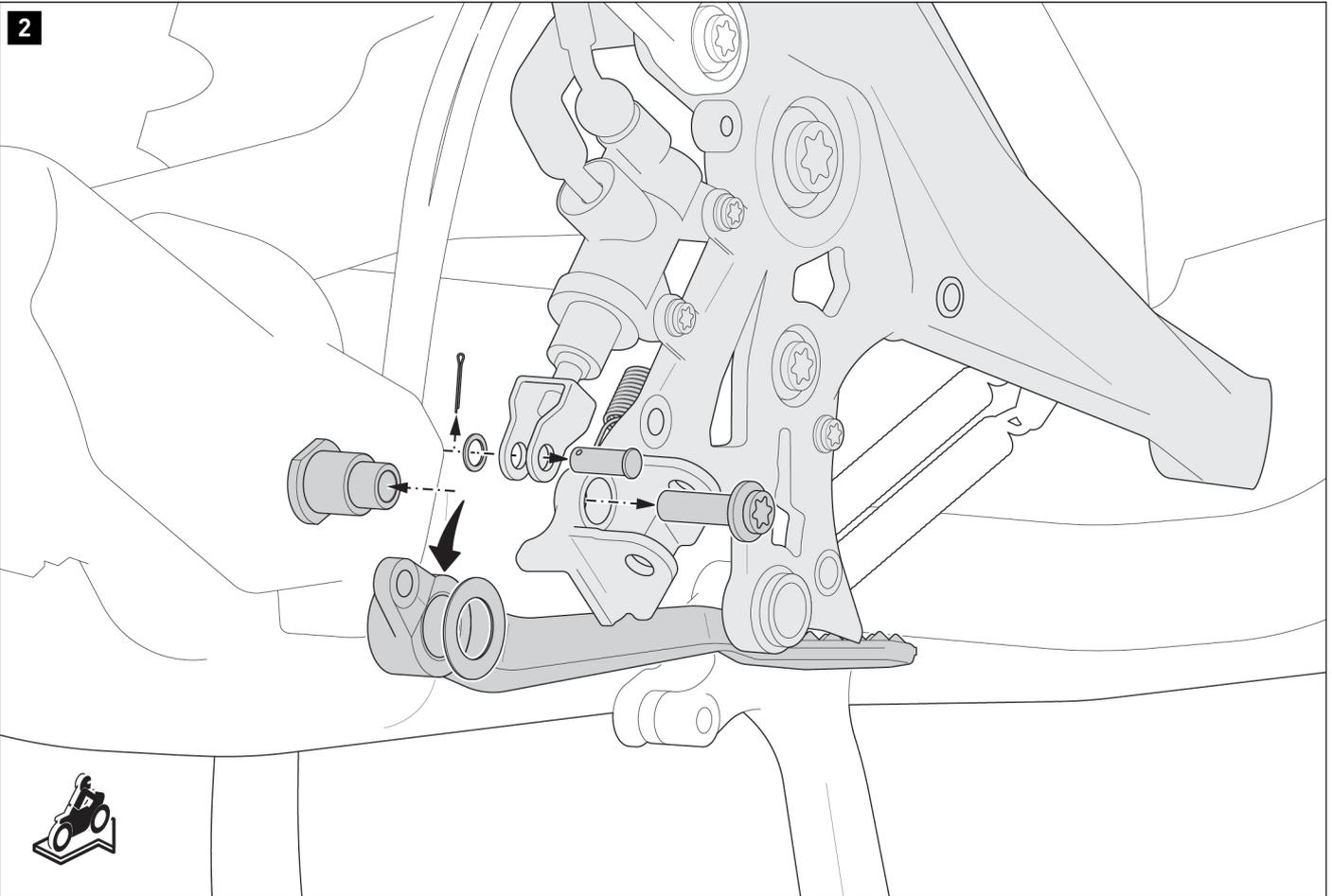
Remove the cotter pin, and loosen the bolt from the master brake cylinder. Loosen the original screws from the footrest mount. Release the springs from the brake lever. Then remove the original brake pedal from the footrest mount.
