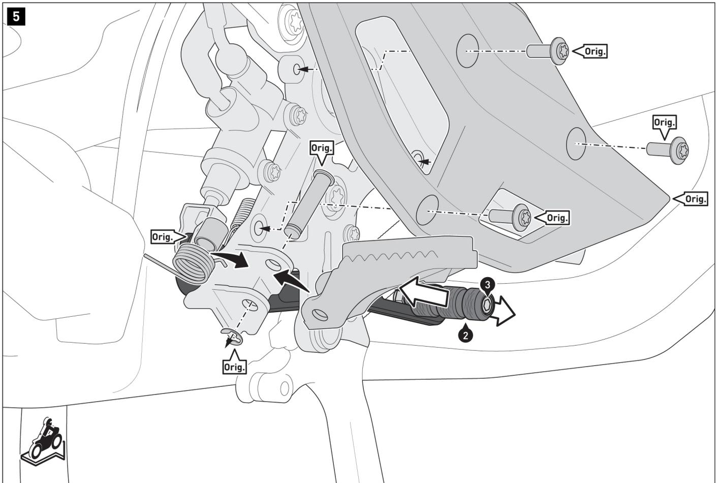
Attach the original footrest with the associated parts to the footrest mount.
