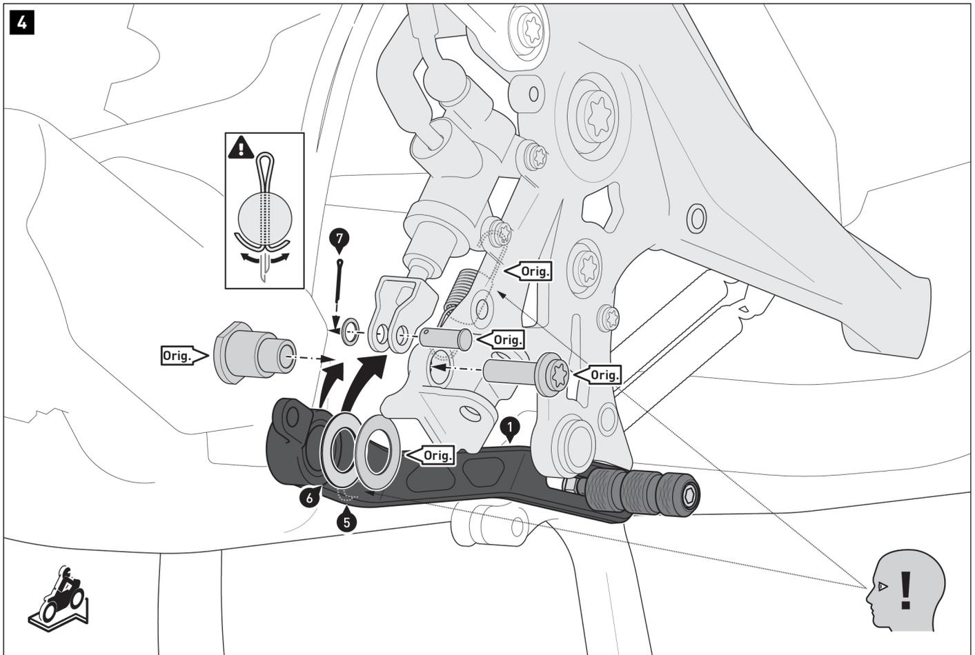
Screw the brake lever to the vehicle using the original parts (Orig.).
