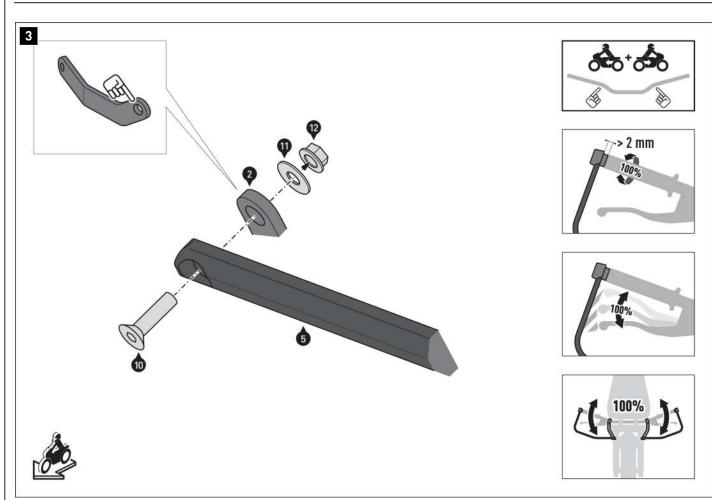
Screw the inner ends of the brackets (5/6) to the connecting plates (2/3). Do not tighten the screws (10) yet.
