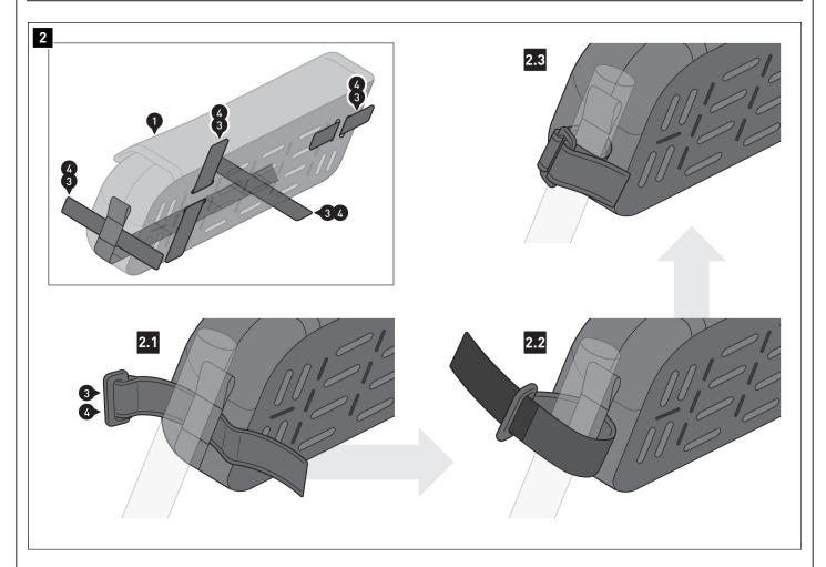
$\triangle$  **NOTE:**The accessory bag (1) can be attached to the vehicle in various positions. The straps (3) and (4) can also be individually attached to the accessory bag (1) in various positions.
