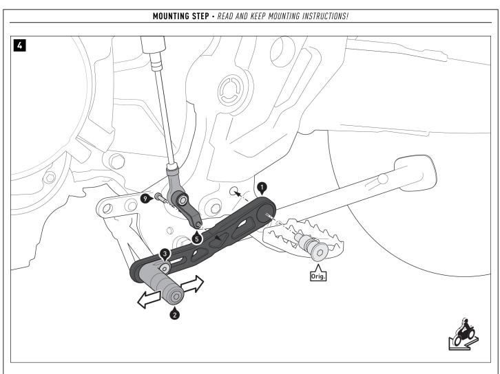
Screw the gear shift rod plate (5) to the gear lever (1). **A WARNING: Use a liquid threadlocker!** Tighten the screw (9) as specified in the mounting instructions.
