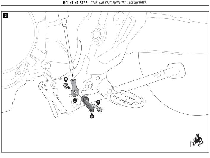
Screw the parts shown together. Then tighten the screw (7) as specified in the mounting instructions.
