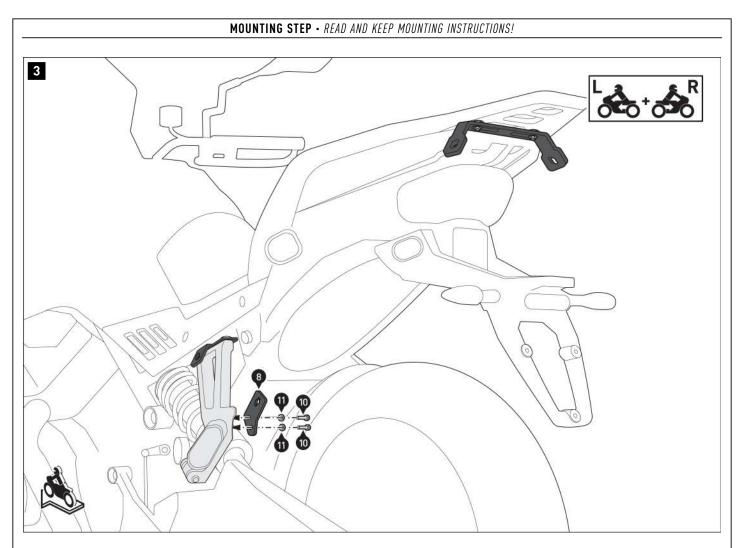
Screw the fastening tabs (8/9) **onto both sides** of the pillion footrest holders. **A WARNING: Use a liquid threadlocker!** Do not tighten the screws (10) yet.
