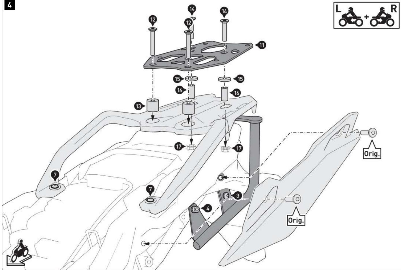
Screw the adapter plate (11) to the original rack.
