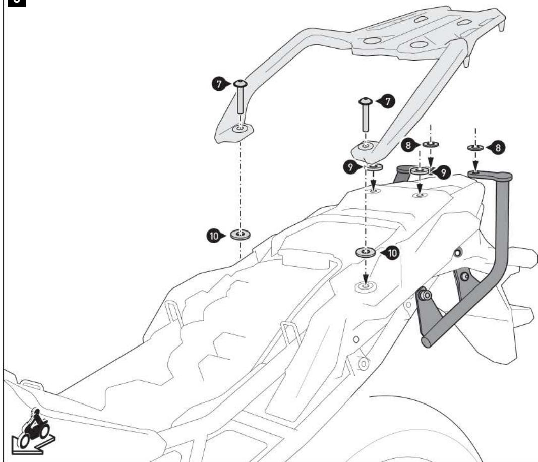
**⚠ NOTE:** When connecting to the SW-MOTECH side carrier, spacers (9) and (10) are no longer required. In their place, mount the side carrier using the parts from the rack.
