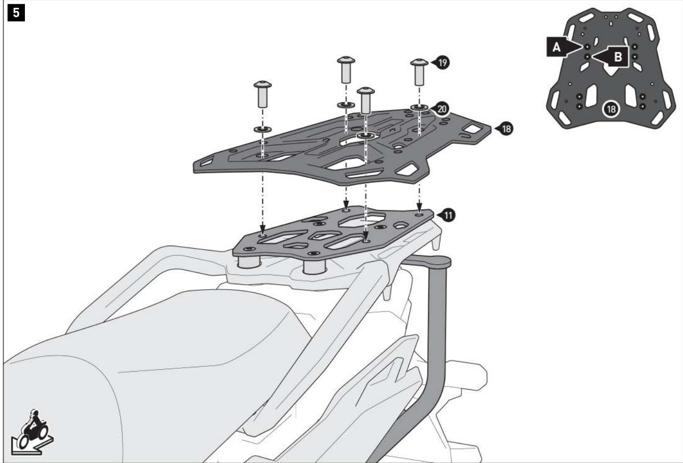
**⚠ NOTE:** Depending on the space available, bolt the rack to mounting position (A) or (B), as indicated in the detailed drawing.
