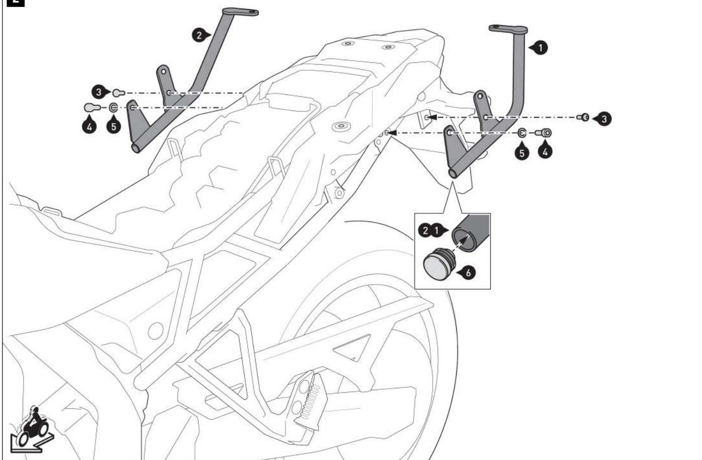
Insert the plastic plugs (6) into the openings on both sides of the side carrier.
